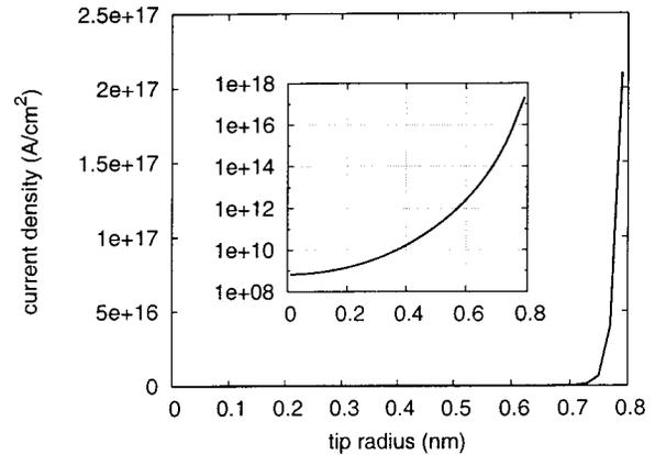
FIG. 9. Emission from the nanotube end along the radius of the tip. The applied field is  $1.4 \text{ V}/\mu\text{m}$ . The inset contains the same data on a log scale, and the units for both views are the same.
