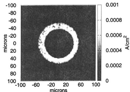
FIG. 10. Current density at the anode for emission from a open-ended nanotube emitting at the tip edge only. The applied field is  $1.4 \text{ V}/\mu\text{m}$  and the zero datum point is the beam centerline.
