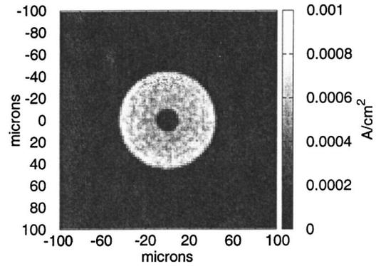
FIG. 6. Current density at the anode for emission from a hemispherical tip emitting between polar angles of  $10^\circ$  to  $50^\circ$ . The applied field is  $1.4 \text{ V}/\mu\text{m}$  and the zero datum point is the beam centerline.
