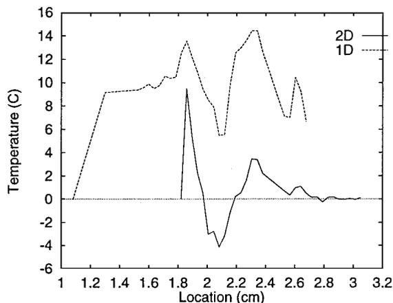
Fig. 10 Residual is the difference between the measured and calculated temperatures for Upilex-2 at 2 s.
