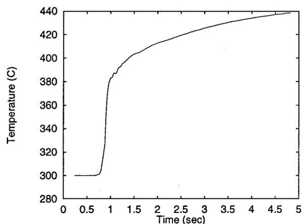
Fig. 4 Temperature response at the sensor of peak heating for Macor-1.
