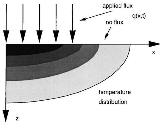
**Fig. 1** Temperature distribution due to a step flux (after some time) indicates that the temperature in the nonheated region will change.
