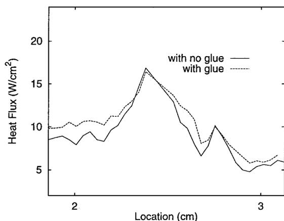
Fig. 9 For Upilex-1 the glue layer was initially ignored and then included in the model.
