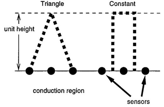
**Fig. 3** Triangular patch provides a linearly varying function in space for sensitivity calculations, whereas the constant patch provides simple implementation but too much bias.
