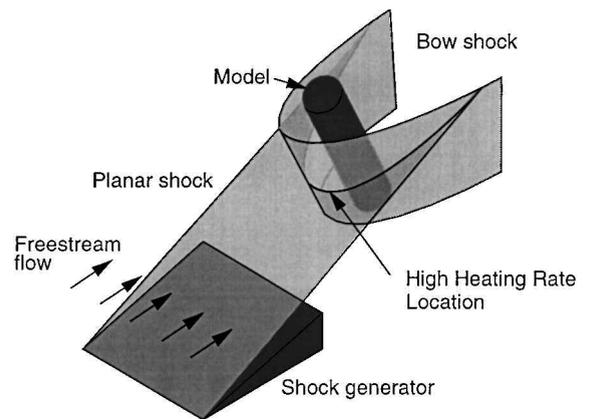
**Fig. 2** Experimental setup shows where the planar shock and bow shock will intersect and produce the high heating rates.
