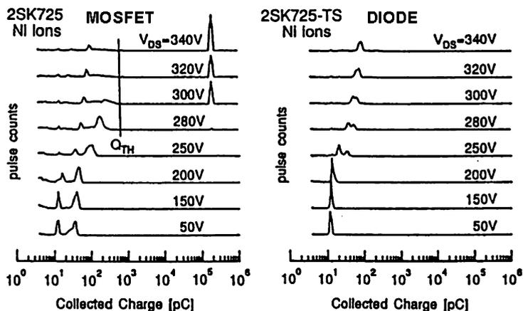
Fig. 1. The collected charge for the MOSFET (2SK725) and the diode (2SK725-TS) when they were exposed to 200 MeV Ni ions (LET=30 MeV/mg/cm<sup>2</sup>) (© 1992 IEEE) [9].
