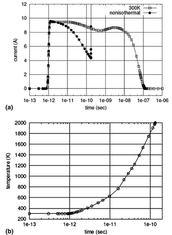
Fig. 9. Output currents of isothermal and non-isothermal simulations with LET = 30 MeV cm<sup>2</sup>/mg and  $V = 3500$  V, along with the maximum temperature due to self-heating [24].
