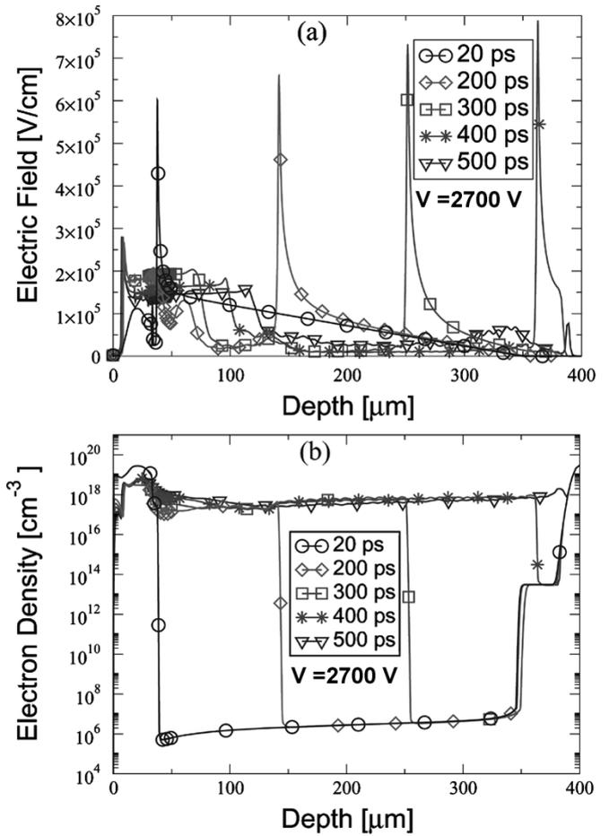
Fig. 8. Spatial and temporal evolution of (a) the electric field and (b) the electron density for an applied voltage of 2700 V.
