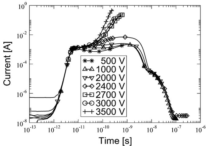
Fig. 10. Nonisothermal simulated output currents at applied voltages of 500 V, 1000 V, 2000 V, 2400 V, 2700 V, 3000 V, and 3500 V.
