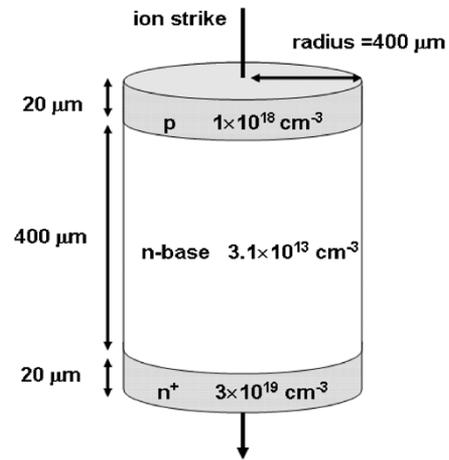
Fig. 3. Power diode structure showing the doping concentrations and the device dimensions.
