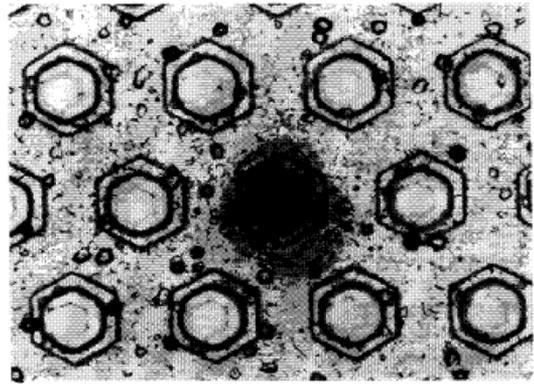
Fig. 1. Optical image of SEB in a power MOSFET (IRF150), after Stassinopoulos *et al.* [2] (© 2000 IEEE).
