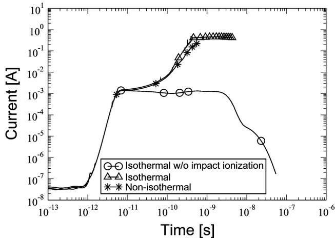
Fig. 4. Comparisons between the electrical characteristics for different models: isothermal, isothermal without impact ionization and nonisothermal simulations.
