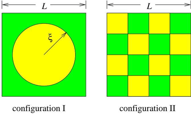
Figure 1. Two-dimensional representation of different configurations considered for effective thermal conductivity calculations. In configuration I, the radius  $\xi$  is varied. In configuration II, the period of the alternating blocks is varied, and mass fraction is held constant.
